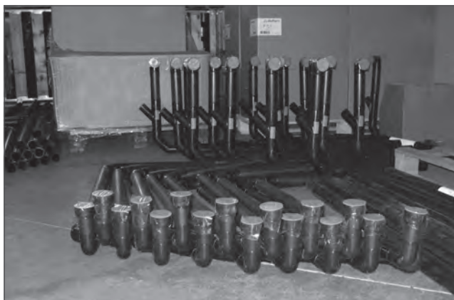
Illustration 9.1 Prefabricated pipe sections
